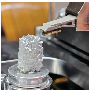
(Figure 1) Cantilever positioned over bone structure.
