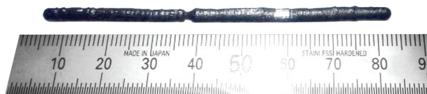
Traveling Solvent FZ (TSFZ) \text{SrCu}_2(\text{BO}_3)_2 could be grown over 320 hrs (14 days) (growth speed 0.25\text{mm/hr} )
